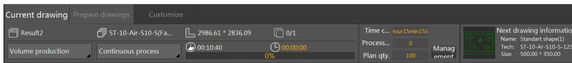
At the top of 《Current Drawing》 is drawing information bar. The message from left to right is: drawing name; technique name; plate size; drawing number; **Volume production** production mode switch; estimated machining time; actual
