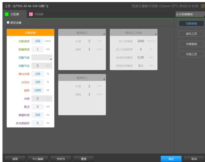
You can check and modify cutting parameter by 'Technique' button. You can click 'Read' at bottom to replace technique parameter from the filter.
