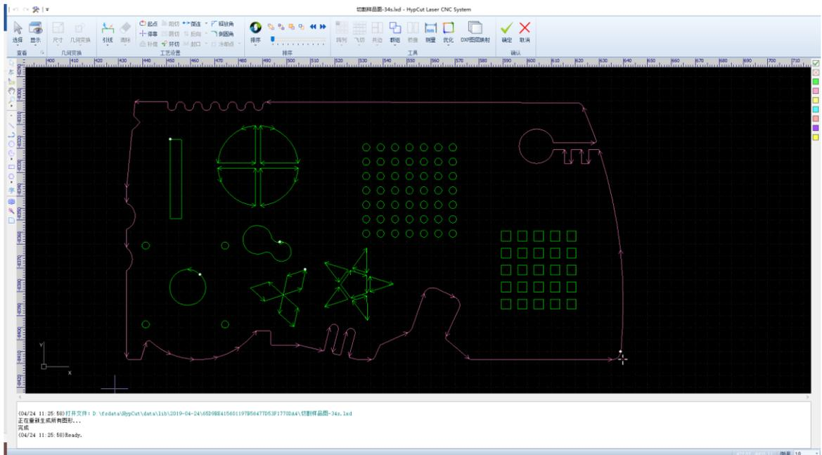
Graphic correction module provides comprehensive CAD edit functions. Details can refer to the related chapter.
