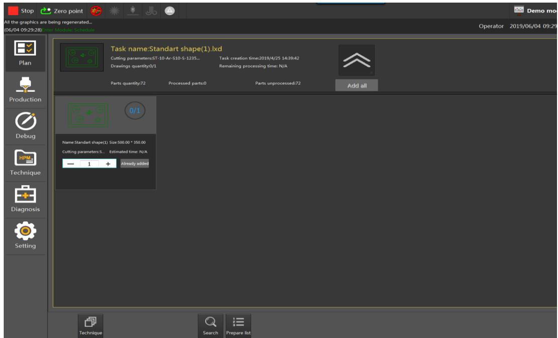
Unfold the task you can see the machining speed, status, parameter setting and add the drawing to the prepare list for machining. You can also edit the graphic or technique of the drawing.
