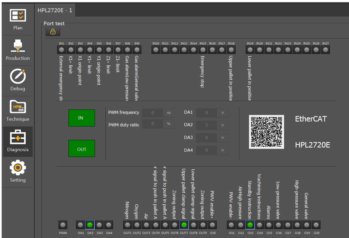
Limit signal used to check if the limit switch well functioned; Monitor the laser emit by PWM signal; There also displayed other 20 input signals and 27 output signals status.
