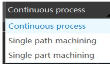
Beside the progress bar is the mode switch of machining process: The default setting is continuous process, under this mode system will stop after whole drawing completed; Under 'single path' mode, system will stop after one single path completed, press continue process next single path; Under 'single part' mode, system will stop after one single part completed, press continue process next part. This function is for cutting technique adjust or exhibition demonstrate.
