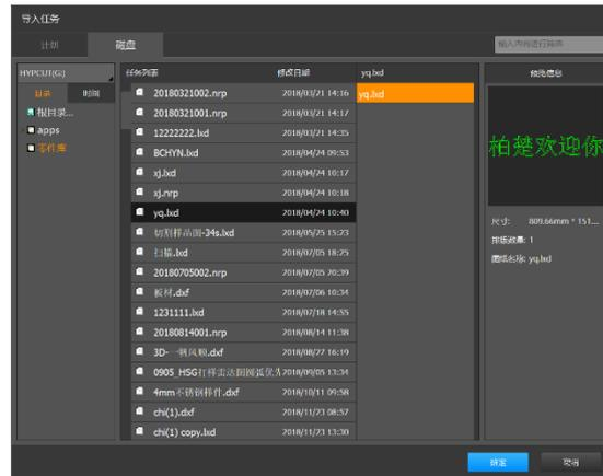
Note:① Volume production only supports nrp, lxd and lxdx formats; Flexible production additionally supports dxf, nc file.
