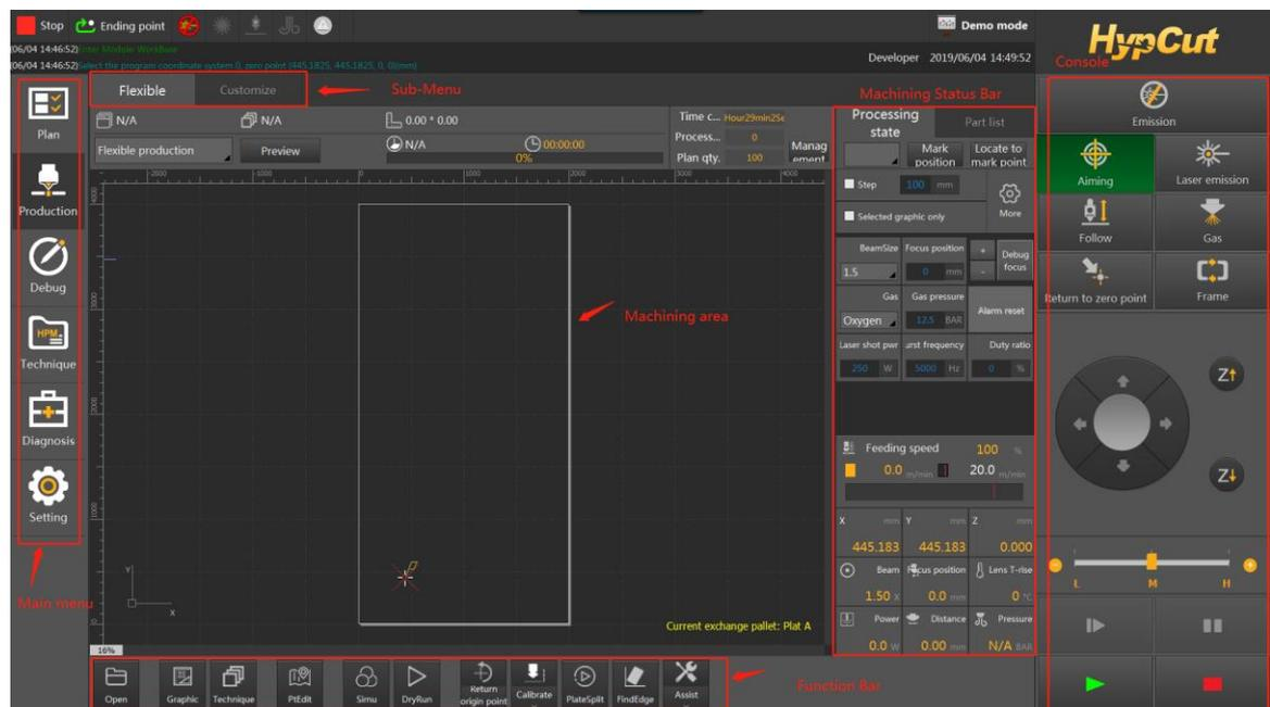
The center zone in black is the graphic display area, the white frame is the machine working frame.
