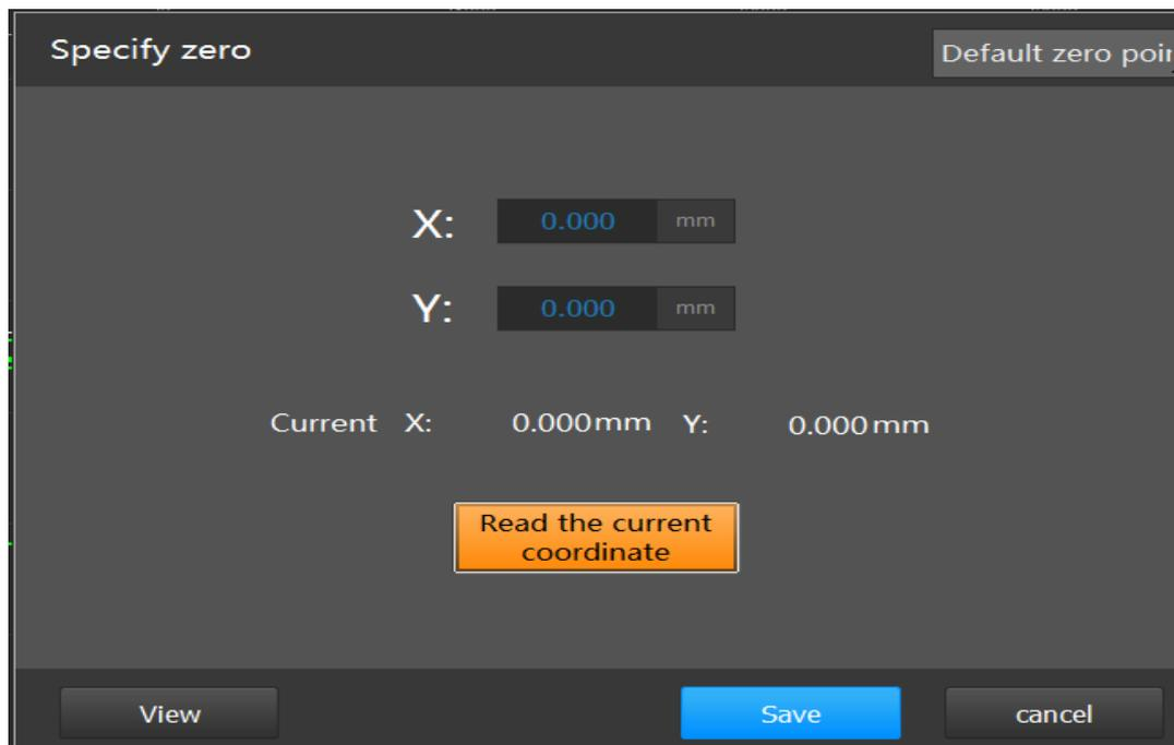
You can enter a specified coordinate or move laser head to any position fit to start production then set as a zero point for production.
