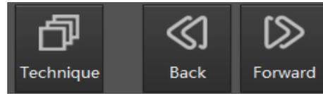
**Backward:** When pause the machining, click the button to move back along the cutting path;
