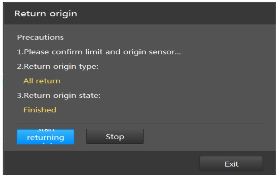
Note: When there are other alarms exist when start the program cannot execute return origin. Only after other alarm removed can execute return origin.
